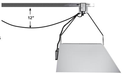
at least 12 inches distance from the bottom of the rail to the center of the power cords arc when the cords are fully extended. Fasten both cords to the bottom of the Drive Motor. You can fasten to either of the two holes or the eye screw described earlier. Please do not fasten to the Motor's Wires.
